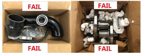
The wheel hubs damaged each other as they bounced around. The uppipe had damage from the clamps flying around in the box and scratching the finish.
